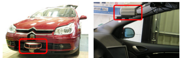
Fig. 7. Experimental platform: Lidar (left), Camera (right)
